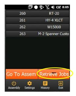
2. Tap on the torque assembly job you wish to open and tap GO TO ASSEMBLY to begin the data collection.
