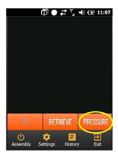
2. Tap the Pressure Setting Input Box. Type in the required pressure and tap ADJUST.
