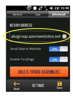
NOTE: It is imperative that the WEB API ADDRESS be correct for complete and proper communication to and from your COMMANDER CLOUD.
