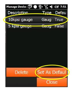
The Bluetooth device you wish to use can be changed for each job simply by selecting a different device and setting it as default. The Default will change from False to True for the new device.
