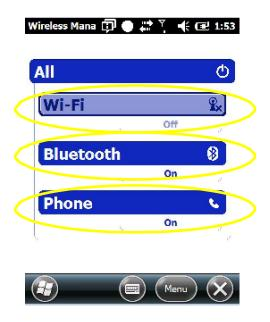
If the Commander is having trouble communicating to Pressure Gauge or Control Module, be sure Bluetooth is turned on.
