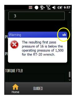
4. If the resulting torque is above the recommended torque by the wrench manufacturer, the system will present a warning message. It will not allow you to proceed.
