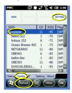
4. Tap the SSID you wish to connect with then tap **SETTING** to input the password.
