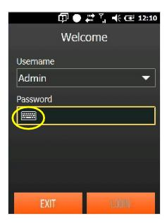
The keyboard at the beginning of an Input Box indicates a virtual keyboard is available. The information can be typed using the keyboard on the COMMANDER or tapped in using the drop down keyboard and stylus.
