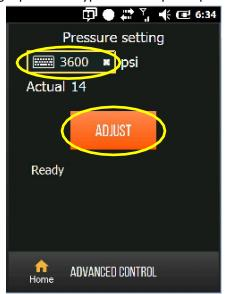
The Pump Pressure will be adjusted automatically. When the pressure is reached, tap HOME
