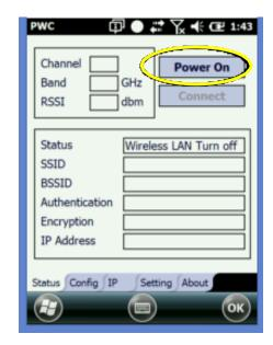
3. Tap the **CONFIG** tab at the bottom and **REFRESH** to identify the available Wi-Fi signals in your area.
