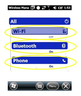
If the Commander is having trouble communicating to Pressure Gauge or Control Module, be sure Bluetooth is turned on.
