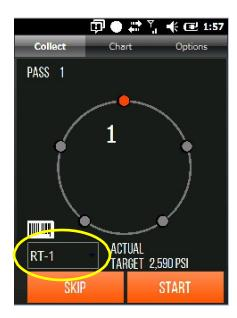
2. By tapping on the Torque Wrench Input Box, a drop down menu of all of the available Torque Wrenches will appear. Scroll through the list and select the correct one.
