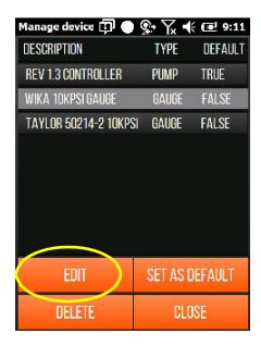
The Edit Device screen appears allowing you to change the description of the device as it appears on the Manage Device screen. You can also change the device type whether it is a pressure gauges or a pump controller.
