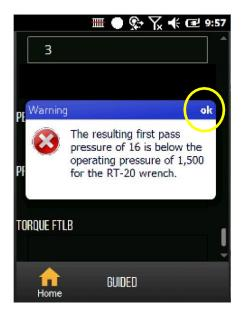
4. If the resulting torque is above the recommended torque by the wrench manufacturer, the system will present a warning message. It will not allow you to proceed.
