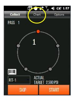
The Torqueing data, taken thus far in the job, will be displayed by pass. The torque or the pressure data can be displayed for the vertical axis. Simply tap the screen to toggle between the two.
