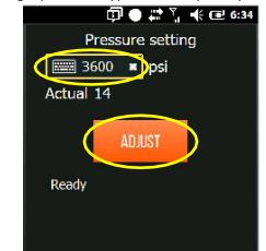
5. Tap the Pressure Setting Input Box. Type in the required pressure and tap ADJUST.
