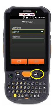
A virtual keyboard is available by tapping the OK button on the handheld while in a window. The information can be typed using the keyboard on the COMMANDER or tapped in using the virtual keyboard and stylus. Tap the OK button again to make the keyboard disappear.
