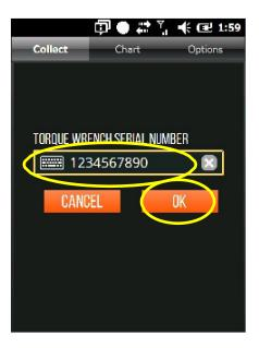
Note: The COMMANDER will warn the operator if the target pressure is outside the range of the Torque Wrench selected and will not permit them to continue until a suitable wrench is selected.
