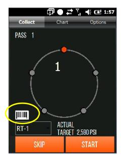
4. Tap on the Serial Number Input Box. You can scan the barcode label on the tool using one of the three orange buttons on the COMMANDER or type the number by hand. Tap **OK** to continue.
