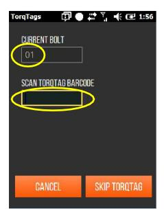
The COMMANDER tells you the correct bolt number in the sequence and compares the barcode scan to verify the wrench placement.
