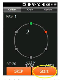
Tap SKIP to move to skip this bolt and move to the next bolt in the sequence. Continue, repeating steps 4-5, until all bolts are tightened for each pass.
