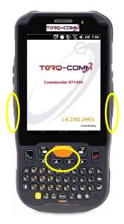
3. If the TorqTag does not match the bolt sequence, you will be instructed to move the wrench to the correct location.
