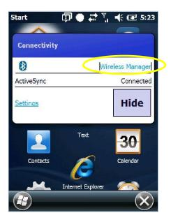
4. From the Wireless Manager screen, you can turn On and Off each of the functions simply by tapping the Input Box. The function will toggle On and Off and the block fade or darken with each tap.
