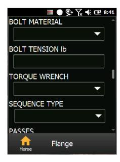
Tap **CALCULATE** to determine the percent yield, final pressure and final torque.
