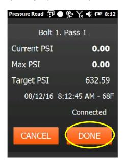
The Collection screen will highlight the next bolt to be tightened. The current bolt is highlighted in RED and the completed bolts are highlighted in GREEN.
